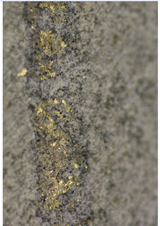
Creso Resources – Visible gold mineralisation in drill core
